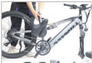
Open the clamp and put the stem into the tube
