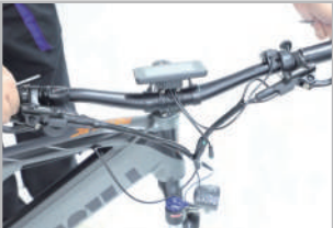
Put the handlebar on the stem
