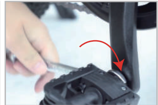
Rotate clockwise to tighten
