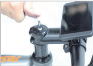
Screw on and tighten
