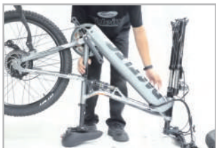
Install the front wheel into the fork
