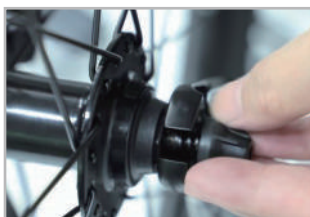
Both sides must be tightened
