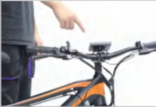
Put the handlebar on the stem
