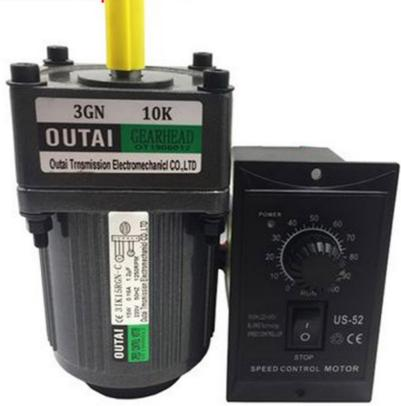
For this speed controller, the applicable motor must be 5 wires, 2 of which are speed feedback. Without these two lines is unable to adjust the speed, and the speed is not stable
