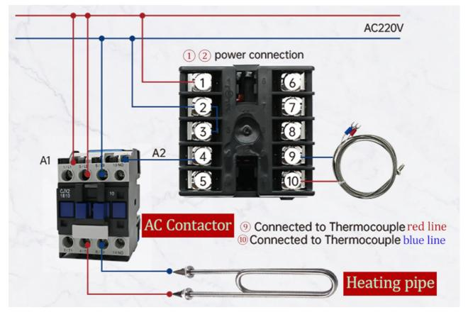
**Note:** The thermal resistance (PT100/Cu50) has three wires, the red wire is connected to 8, and the other two wires are connected to 9 and 10 at will.
