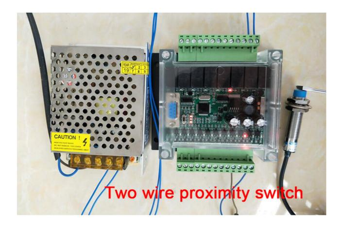
PLC wiring diagram as above (XC is 0V)
