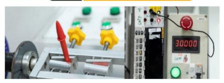
The 8KV High Voltage Impact Test Lasting 1 Minute, 5000 Swing Tests, And 30,000 Plug-In Tests Ensure The Safety And Durability Of The Test Leads!
