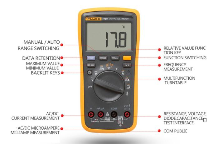
\*THE TEMPERATURE, FREQUENCY, RELATIVE VALUE FUNCTION KEYS ARE 17B+ UNIQUE
