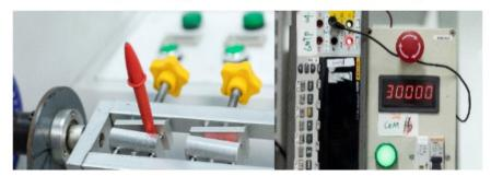
The 8KV High Voltage Impact Test Lasting 1 Minute, 5000 Swing Tests, And 30,000 Plug-In Tests Ensure The Safety And Durability Of The Test Leads!
