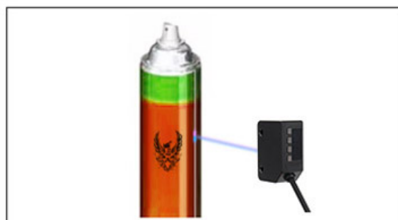
Detecting gaps in spray cans
