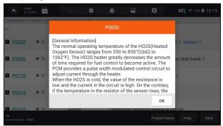
Figure 5-12 Sample DTC Help Screen
