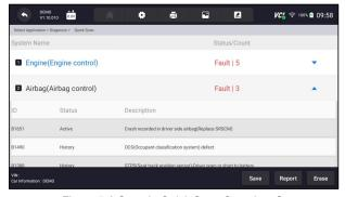
Figure 5-3 Sample Quick Scan Complete Screen
