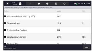
Figure 5-11 Sample Freeze Frame Screen
