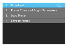
In the submenu, 16 preset parameters can be saved, and every preset parameter includes all parameter information of source setup (signal source, PIP, scaling, cropping, picture adjustment), users can also directly load the saved preset parameter to display the image according to needs, and don't need to set up all parameters again.
