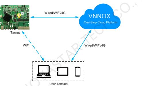
VNNOX could be accessed directly or by way of bridge connection. When bridge connection is selected, the following three methods for Internet connection of Taurus products are available with priorities ranging from high to low:
