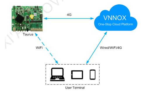
VNNOX could be accessed directly or by way of bridge connection to centrally manage post screens. Taurus products can connect to the Internet through the wired network, Wi-Fi and 4G network which is recommended for this solution.
