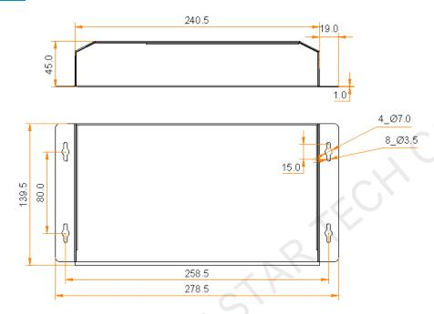
Tolerance: ±0.1 Unit: mm
