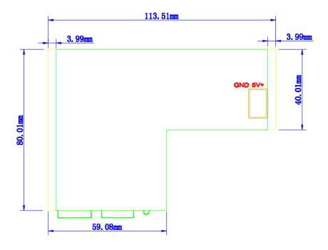
Fig. 2 CVT320 internal dimensions
