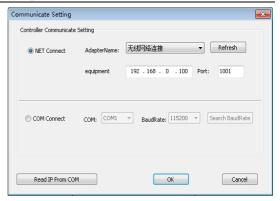
This software has "Net Connect" and "COM Connect" available; when different "Connect" modes are selected, different preparations will be necessary.
