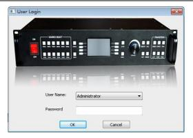
For the first use, there is no password so just click "OK" directly; if a user password has been set, the software control/setting will not be accessible unless the correct password has been entered.
