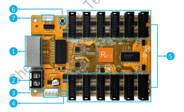
①: Gigabit Ethernet port, used to connect the sending card or receiving card, the same two network ports are interchangeable,
