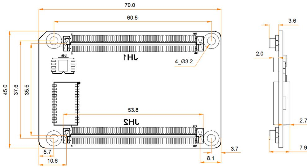
Tolerance:  $\pm 0.1$  Unit: mm
