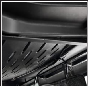
Ventilation slots for preconditioned seating
