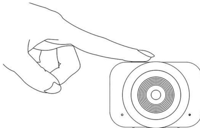
**Power Button:** Press and hold the power button for 4-5 seconds to turn on the camera when it's off.
