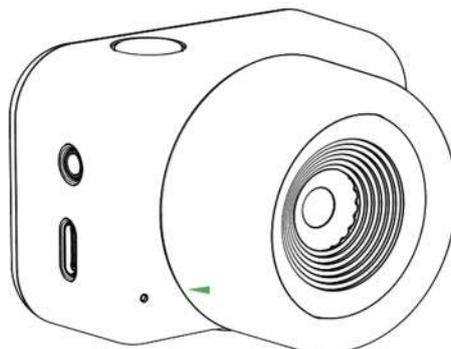
The camera is set to focus on objects beyond 80cm away when the focus ring is in the preset position (green focus mark aligning with the status LED). Rotate the focus ring counter-clockwise steadily to set focus on objects ranging in between 7 to 80 cm away until the image is sharp.
