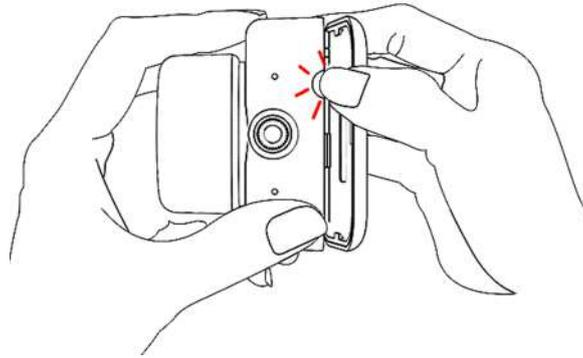
b. Insert the battery as shown below.
