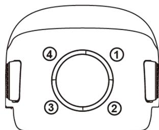
When the battery is turned off, press the power button for 1 second and then release it quickly to check the battery level. LED will indicate the current battery level, as shown below.
