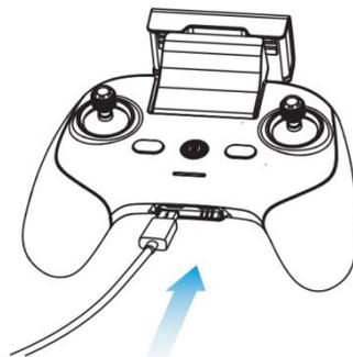
2. In the case of charging, the power indicator of the remote controller will enter the mode of waterfall light. After completion of charging, the four indicators will be normally on green. At that time, you will hear two beep sounds.
