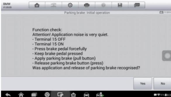
**Figure 5-7 Sample Parking brake: Initial operation**
