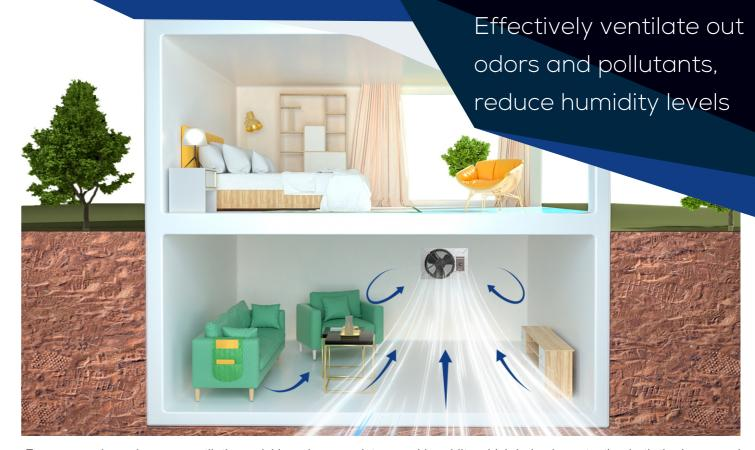
Fan-powered crawl space ventilation quickly reduces moisture and humidity which helps in protecting both the home and the occupant. This crawl space fan increases air circulation to fight condensation and ventilates excess moisture which can be the cause of mold, mildew and wood rot. The constant operation of this unit helps vent radon, treated wood off-gassing and odors that might otherwise migrate into the living spaces of the home.
