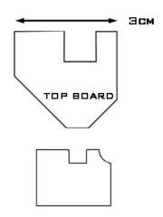
4. Paste the PVC stickers on the surface of DTU PCB to prevent electric leakage.
