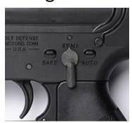
27. If you only get a SAFE function and a SEMI-AUTO function without FULL-AUTO function after the gearbox is installed into the receiver, the position of the white sticker on the selector plate should be not correct, it indicated that the full-auto sensor can not be activated when the selector plate is in the FULL-AUTO position. Move the white sticker to the left 1-2mm until the functions are normal.
