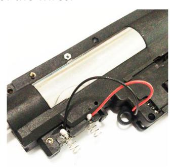
24. After correct installation, when the selector plate is in SAFE position by default setting, the trigger can still be pulled, but the DTU will not react. When the selector plate is in SEMI-AUTO or FULL-AUTO position, the DTU will react.
