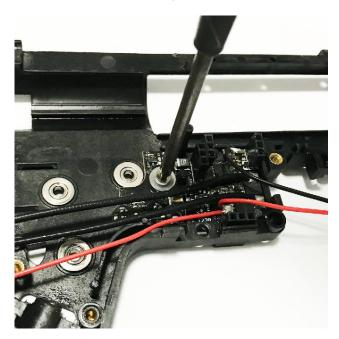
13. Adjust the wires, make sure that the sensors' surface are clean and not blocked.
