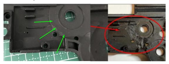
16. Check whether the top board can be leveled against the gearbox. If not, it is recommended to modify the gearbox first.
