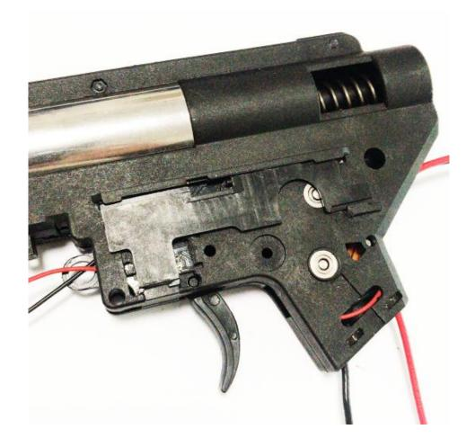
23. If you are using a gel ball gearbox, solder these two wires and pay attention to the order of the wires.
