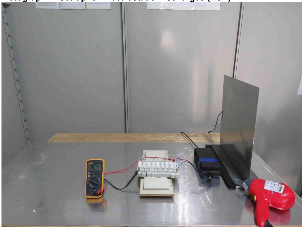
Photograph 7: Set-up for Electrostatic Discharges (ESD)
