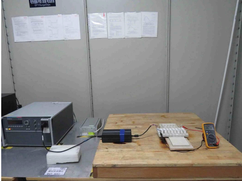
Photograph 4: Set-up for EFT
