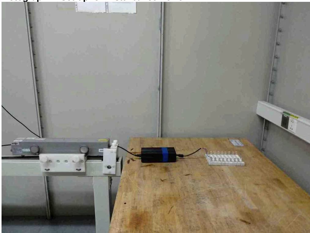
Photograph 2: Set-up for Disturbance Power
