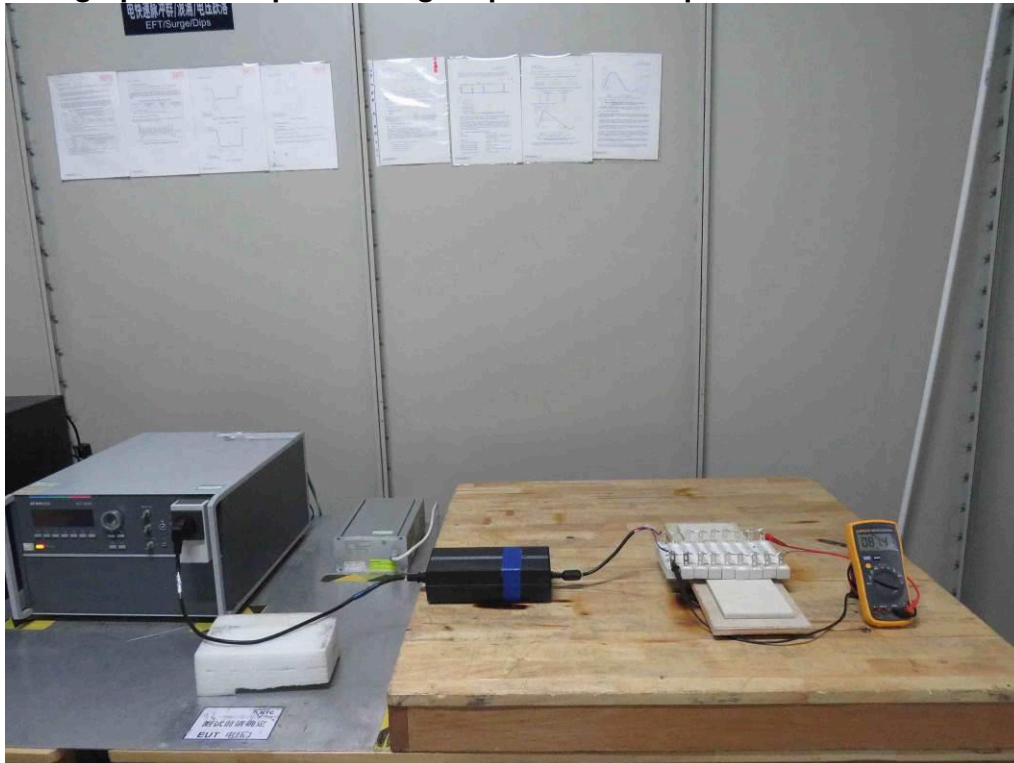
Photograph 6: Set-up for Voltage Dips and Interruptions
