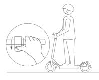
When the scooter starts to run, put the other foot on the pedal, and then press the acceleration button (when the scooter accelerates to more than 3km/h); to decelerate, release the acceleration button. The energy-saving mode is turned on when the scooter starts to slow down. To brake, pinch the brake lever on the handlebar.
