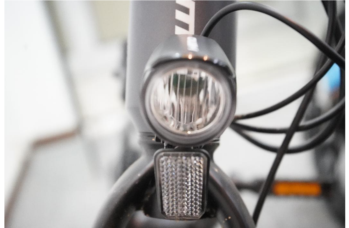
Z20 Max headlight with reflector passed E-Mark certificate
