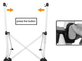
**2** Press in the upper part of the button and push the frame in until it's fully closed.
