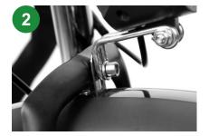
Remove the screw from the front fork. Screw as shown in the picture through the gasket, headlight, fender to assemble.
