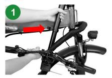
Open the quick release on the standpipe. Thread the handlebar into the standpipe.
