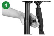
Raise the handlebar to your preferred height. Press quick release, lock the handlebar.
