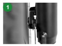
Attach the tire to the front fork. Make sure the brake disc goes through the gap in the middle of the brake
