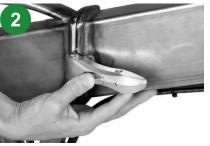
Hold the push button with your right thumb. Release your left hand. With the other fingers of the right hand, open the fold from the bottom
