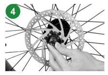
Remove the nuts and water drop gaskets on both sides of the front wheel.
