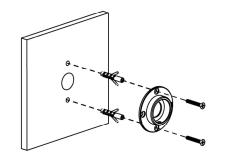
Choose the appropriate drilling location to fix the Base on the wall with a drill and a screwdriver.
