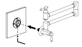
Wrap the PTFE tape onto the adapter, screw the Tap body to the proper position, then lock the hex socket screws with a Hex key.
