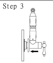
Open the Tap for water flow and check if any leakage. Finally, press the decorative cover tightly to the wall.
