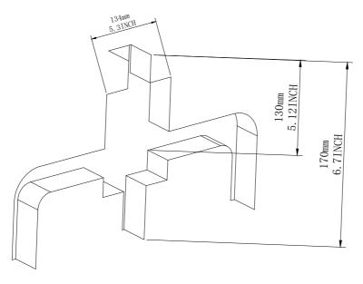
2. The depth of the embedded box is 2.36  $^{\bullet}$  - 3.15  $^{"}$  It's better to drill the depth of 2.36  $\!\!\!\!$  for blank wall
