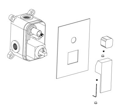
According to the figure below , please correctly adjust the direction of water separator handle
