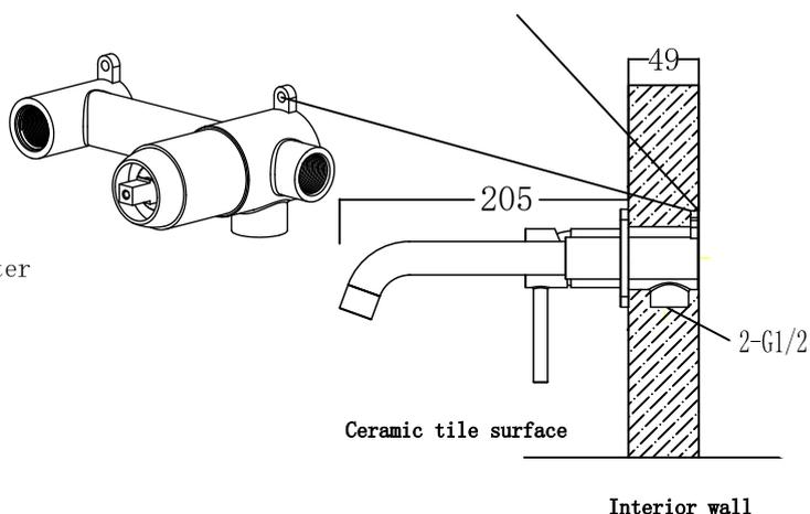
PS: In the process of embedding the wall, please do not remove the protective sleeve to avoid damaging the copper sleeve.
