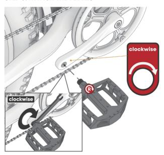
Insert the right pedal ("R" sticker) into the right crank's threaded hole and rotate the pedal (clockwise) until some tension is felt.
