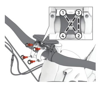
Remove the handlebar clamp from the stem by removing all screws with the M5 hex key. Insert the handlebar into the stem and reinstall the clamp. Make sure the handlebar is aligned with the front wheel before tightening and the stem is not set above the maximum height indicator.
