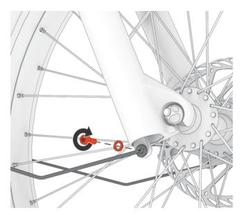
Unscrew the bolt first. Connect the fender struts with the fork by tightening the screws and flat washer clockwise with the M4 hex key.
