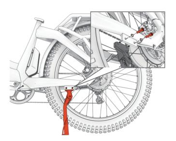
Open the shipping carton and carefully remove your bike from the bottom tray. Kickstand comes with 2 bolts. Remove the 2 bolts from the kick-stand with the M4 hex key. Put the kickstand under the bike and align the holes on it with the holes on the bike. Then thread the bolts into the holes and tighten them with the M4 hex key.
