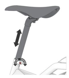
Loosen the adjustment bolt of the seat clamp, insert the seat tube, then lock the adjustment bolt after adjusting to the appropriate height.
