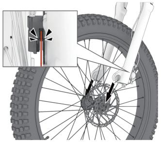
First, remove the brake protection plate, and slide the front wheel into the front fork, so that the disc brake is inserted into the center of the brake caliper, while the front hub axle is stuck into the front fork slot.
