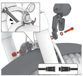
Unscrew the nut and gasket from the end of the long bolt and make sure the headlight bracket is on the outside of the frame and the fender bracket is on the inside. Align the holes on the two brackets to the hole on the fork crown. Pass the long screw through the holes. Tighten the screwed nut from the end of the long screw with the M5 hex key and 10mm open wrench.
