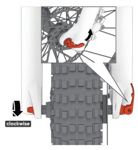
Move the quick-release lever into the open position. With one hand on the quick-release lever and the other on the adjustment nut, hand tighten the adjustment nut until you start to feel some resistance against the fork.
