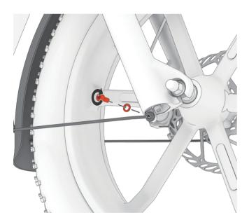
Unscrew the bolt first. Connect the fender struts with the fork by tightening the screws and flat washer clockwise with the M4 hex key.
