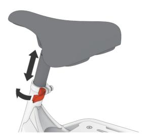
Unlock the quick-release lever and insert the seat post into the seat tube.
