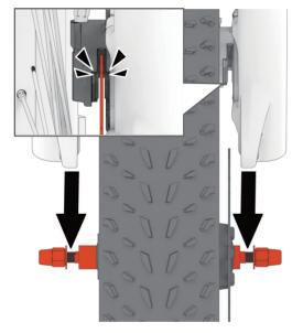
Slide the wheel into the fork dropout slots. Insert the disc rotor into the center of the disc brake at the same time you are inserting the wheel axle into the fork drop out. Make sure that each fork drop out should be placed between the flat washer and the fender washer.
