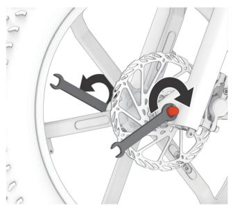
Use two 15mm wrenches to tighten axle nuts on both sides of the wheel to 20–25 NM at the same time.
