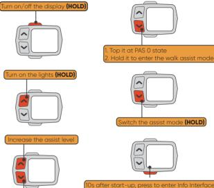
10s after start-up, press to enter Info Interface Within 10s of start-up, hold to enter Option Interface 10s after start-up, hold to enter Clearance Interface
