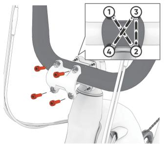
Remove the handlebar clamp from the stem by removing all screws with the M5 hex key. Insert the handlebar into the stem and reinstall the clamp. Make sure the handlebar is aligned with the front wheel before tightening and the stem is not set above the maximum height indicator.
