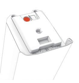
If you use the battery for the first time or do not use it for 15 days, press and hold the battery wake-up button for more than 10 seconds to activate the battery until the indicator next to it flashes.
