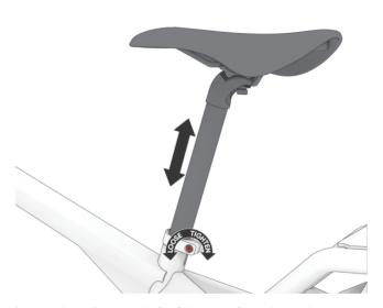
Loosen the adjustment bolt of the seat clamp, insert the seat tube, then lock the adjustment bolt after adjusting to the appropriate height.
