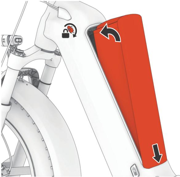
When installing the battery, first insert the low end of the battery into the internal slot of the downtube to ensure that the terminals at the bottom of the battery are smoothly inserted into the slot inside the downtube. Then push the upper end of the battery into the downtube and turn the key to the right to lock it.
