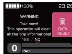
After data clearing, the TRIP distance, average speed, maximum speed, and Assist Mode usage statistics return to zero. The TOTAL distance data (ODO) can not be cleared by
