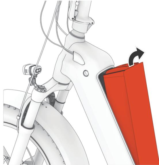
As shown in the picture, carefully remove the battery.
