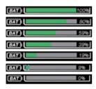
The power bar flashes when the battery level is 0
