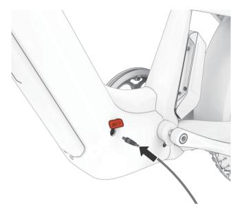
Open the charger cover. Insert the charger probe into the charger port. Make sure the connector is free from dirt, and debris, and dry before connecting the charger to the battery.
