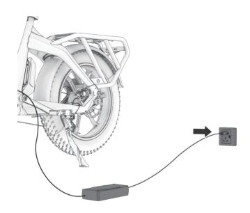
Insert the AC plug into an AC outlet. The red indicator light turns on and will remain red until the battery is fully charged. The indicator light turns green once the battery is fully charged.
