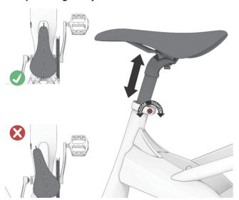
Loosen the adjusting bolt of the seat clamp and adjust the seat tube to the appropriate height. Then lock the seat clamp and make sure the stationary ladle faces forward.
