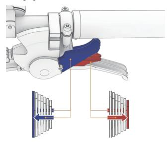
When pedaling, pull the upper lever with your index finger to shift your bicycle into a higher gear (harder/small cog) and push the lower lever with your thumb to shift your bicycle into a lower gear (easier/large cog).
