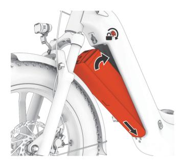
When installing the battery, first insert the low end of the battery into the internal slot of the downtube to ensure that the terminals at the bottom of the battery are smoothly inserted into the slot inside the downtube. Then push the upper end of the battery into the downtube and turn the key to the right to lock it.
