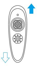
In mode 2, press and hold the gravity unlock key, the remote controller low in front and high in rear will make the aircraft fly forward; the remote controller high in front and low in rear will make the aircraft fly backward.
