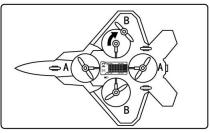
Pinch the small cap in the middle of the fan blade and take out. When replacing, press down on the motor shaft, being careful not to deform.
