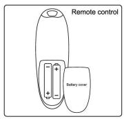
Open the battery cover and install two 1.5V "AAA" batteries (as shown)
