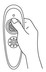
In mode 1, push the joystick of the remote controller forward to fly the aircraft forward; pull it backward to fly the aircraft backward.
