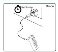
Insert the USB interface of the USB charging cable into the power adapter with an output: 5V=2A. The battery will light up when it is in USB charging and it will turn off when the battery is fully charged. Charging time is about 60 minutes.
