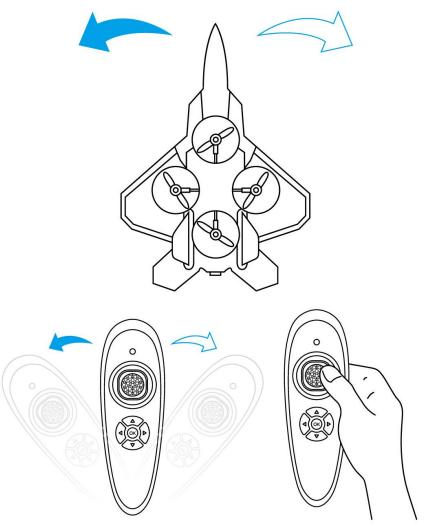
In mode 1, press and hold the gravity unlock key, tilt the remote control to the left to turn its head left; tilt to the right to turn the aircraft's head right.
