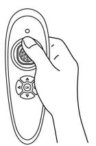
In mode 2, push the joystick of the remote controller forward to ascend the aircraft; pull the joystick backward to descend the aircraft.
