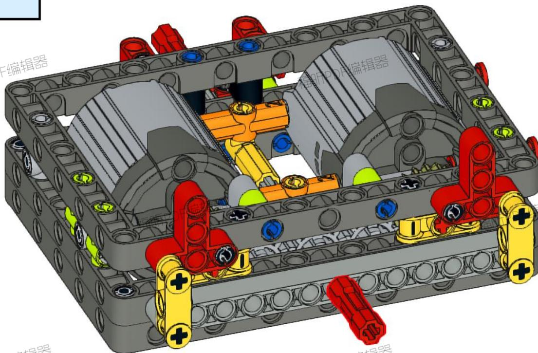
Assemble it here, stack and install the motor wire head on the lithium battery to test whether it can rotate normally, and then continue to assemble
