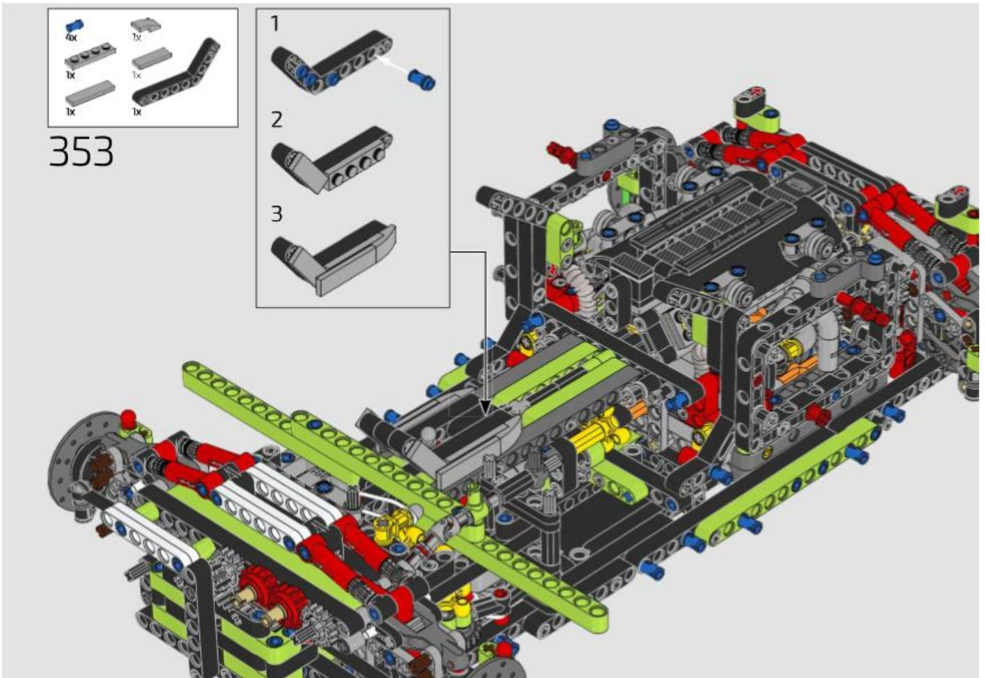
Continue to assemble the whole vehicle according to step 356 of the manual. After that, put the lithium battery in the trunk of the vehicle. Connect the motor connector and **win**
