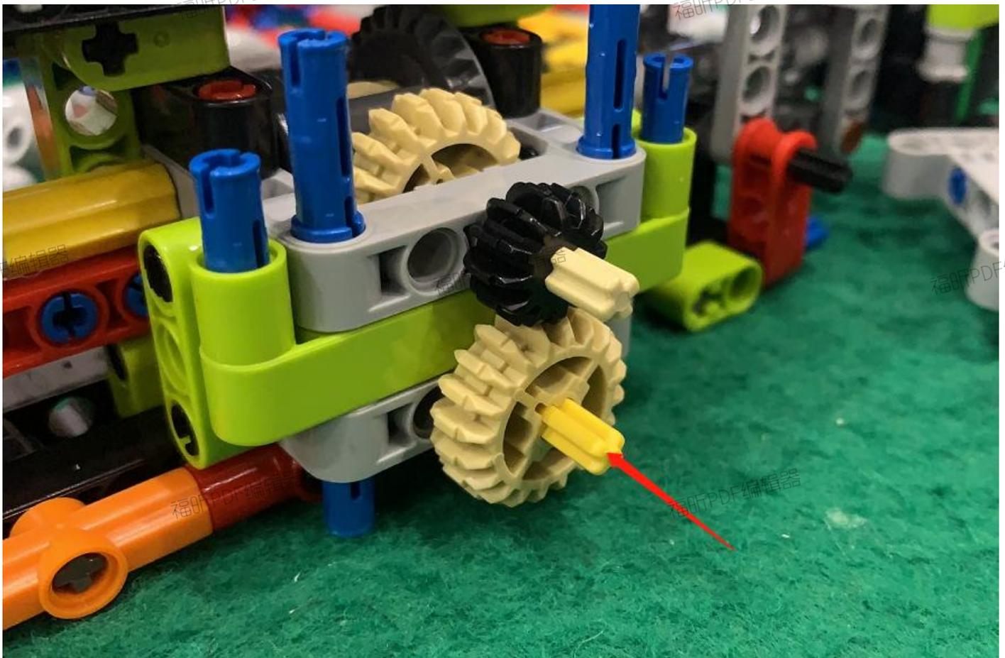
Link the front and rear main bodies, and pay attention to the alignment of the four hole positions!
