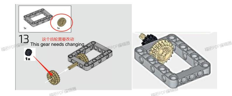
Continue to assemble according to the instructions 14-44, and the changes required in step 45 are as follows:
