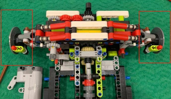
The servo motor can be installed only when both sides of the wheel are parallel and centered, and the cross hole of the gear on the serrated shaft is positive cross!
