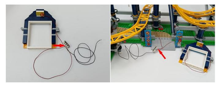
Excessive lighting wire is wrapped around the expansion board.
