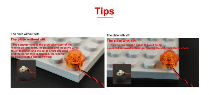
The slit on the the plate round 1X1 are hand-made to avoid squeeze the wire and cause short circuit and abnormalheat during installation.
