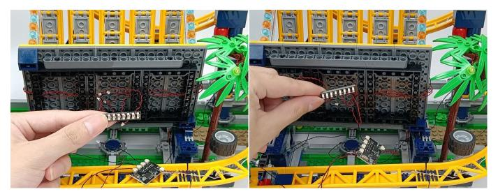
The 5cm cable on the module is connected to the expansion board.
