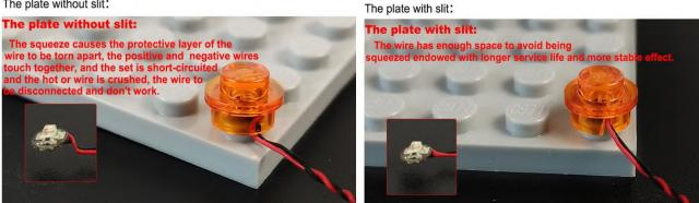
The slit on the the plate round 1X1 are hand-made to avoid squeeze the wire and cause short circuit and abnormalheat during installation.
