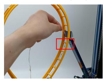
Wrap the remaining lighting wire around the track. The black part of the lighting line is placed in the red box in the picture.
