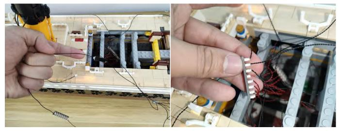
Unplug the 20cm cable on the 8-seater expansion board from the power supply.
