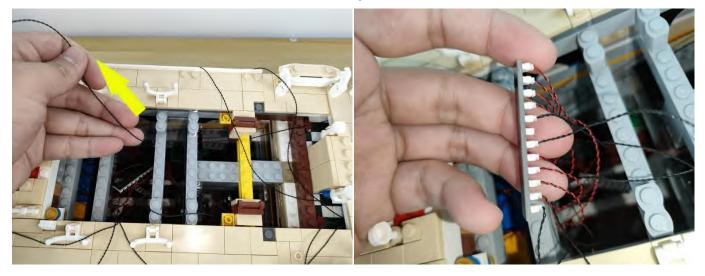
Unplug the 20cm cable on the 12 expansion board from the power supply and place it at the position shown in the figure.
