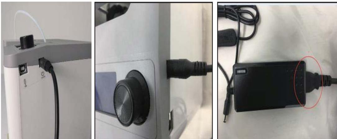
7. Flip the power switch on the inline control to the ON position (I). After the printer finishes booting, you will see the following wizard. Depress the Knob on top of the printer to select Next on the Welcome Screen, then again to select Next on the STEP 1: LOAD FILAMENT Screen.
