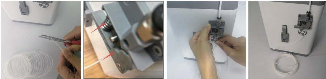
to start the Loading Filament function. The Nozzle will heat to the target temperature, if necessary, then will load the filament and extrude a small amount. Clean the extruded filament.
