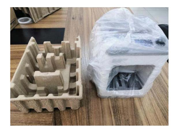
4. Remove the cardboard block from the inside of the printer.
