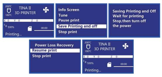
The Tina 2 printer features the ability saving a print in progress, so that you can turn the printer off and resume printing at a later time. Perform the following steps to save and resume a print in progress.
