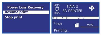
In the event that power is lost for any reason, the printer will remember where it was in the print process when power was lost. Perform the following steps to continue the interrupted print.
