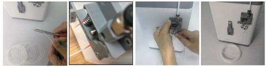
press the Knob again to stop extrusion, then press the Knob to select the Continue option.
