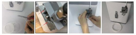
to start the Loading Filament function. The Nozzle will heat to the target temperature, if necessary, then will load the filament and extrude a small amount. Clean the extruded filament.
