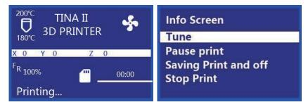
1. With the Printing... Screen displayed, press the Knob to display the Print Control Menu.
