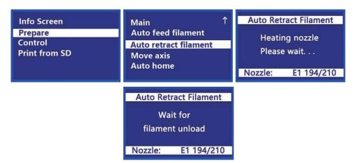
On the Main Menu, rotate the Knob until the Auto Retract Filament option is highlighted, then press the Knob. The Nozzle will heat to the target temperature. Once the target temperature is reached, the Extruder motor will retract the existing filament.
