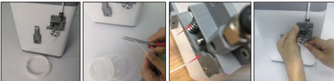
Press the Knob to start loading filament. Once filament starts extruding from the Nozzle, press the Knob again to stop extrusion. Clean the extruded filament, then press the Knob to select the Continue option.
