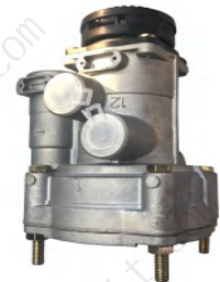
Control Valve, trailer RDA3173151
