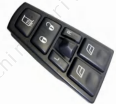
Switch, mirror adjustment drivers door window lift RDA20752918
