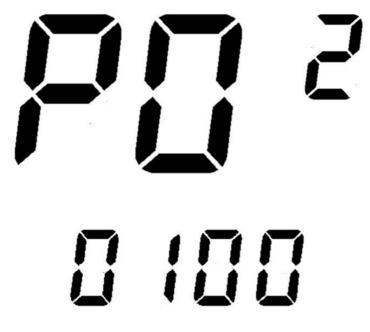
The P02 parameter is used to correct the currently displayed speed value. This parameter works regardless of the phase voltage speed or the Hall speed. The purpose is to correct the current speed display value. The coefficient value is between 0.20-1.50 (actual display 20-150), each time the button jumps the value 5, the actual corresponds to 0.05, the value changes as follows: 10->15->20->....100->105->110->....->150->10
