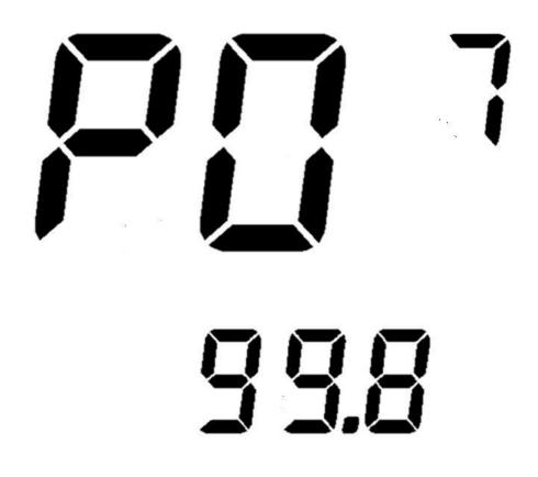
This parameter is similar to the speed coefficient. The customer feedback battery voltage measurement value is not accurate. This parameter is used to correct the battery voltage value. The value of this parameter is from 95.0% to 105.0%, and each press of the button increases 0.2%.
