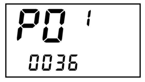
When the lower number is flashing, press the button to select the actual value of each parameter:
