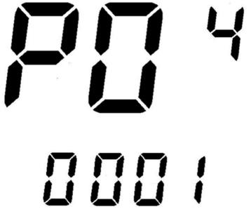
P04, 1 represents the phase voltage speed measurement, 2 represents the Hall speed measurement. This parameter is used to distinguish the phase voltage speed measurement and the Hall speed measurement parameter. When the phase voltage is measured, the subsequent wheel diameter and magnet steel parameters will not work.
