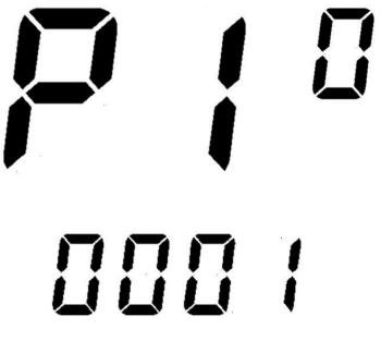
P10 is the unit of speed mileage, 1 for kilometers, 2 for miles, default is 1 Note: Speed, single mileage, cumulative mileage units need to be switched according to this parameter
