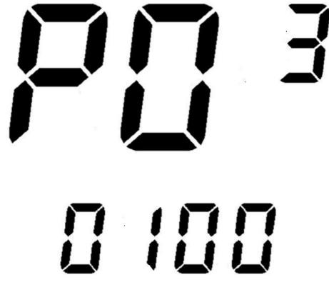
P03, because the battery life is sensitive, the OEM may need to manually enlarge the mileage data. This parameter is used for this purpose. The parameter can be between 1.00-1.30 (display 100 to 130), and each time the button is pressed, 5 is added. (actually 0.05), 1.00->1.05->1.10->1.15->.1.20->1.25->1.30->1.00, multiply the currently displayed mileage (single and cumulative) values by this parameter. Get the displayed mileage of the virtual standard.
