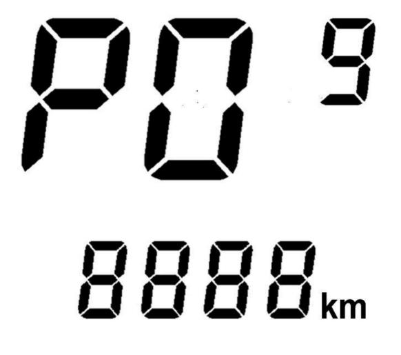
After entering the PO9 parameter, press and hold the (>3 seconds) button to accumulate the mileage. At this time, press the button 10 times continuously to clear the accumulated mileage.
