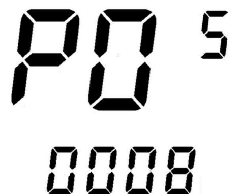
P05 is the rim size, you can choose the rim diameter: 8 inch, 10 inch, 12 inch, 14 inch, 16 inch, 18 inch, 20 inch, 22 inch, 24 inch, 26 inch, 28 inch, 29 inch (phase voltage Does not work when measuring speed), the default value is 14 inches
