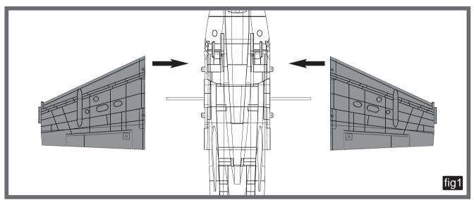
3.Secure the left and right wing to the fuselage using the 4 screws included (fig2)
