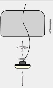
1. Put the gasket on the LED bulb then tighten it.
