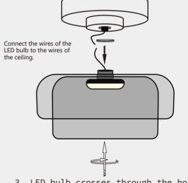
3. LED bulb crosses through the hole of the first large shade then with the third gasket tightened.
