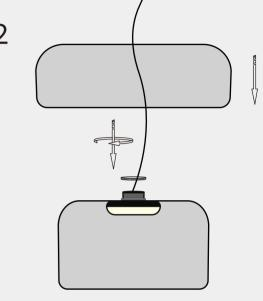
2. LED bulb crosses through the hole of the second layer shade, put the second gasket then tighten it.
