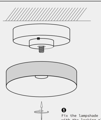
Fix the lampshade with the locking plate.
