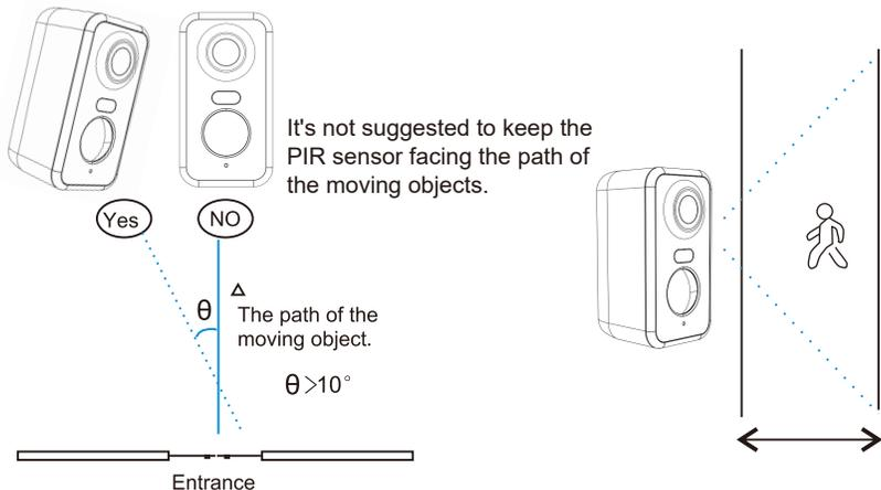
When installing the camera, the PIR sensor should not be vertically aligned with moving objects, as it may not detect movement. It is recommended that the camera be tilted at more than 10 degrees to capture all motion.
